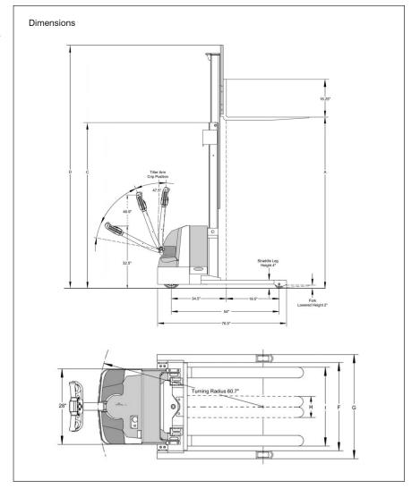
Note: Aisle dimensions listed above assume the bay width to be straddled OD plus 2" (1" on either side of straddle leg). Straddle OD is the load width plus 8". \*For metric conversion multiply inches by 25.4.
