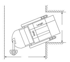
**Note:** Aisle dimensions listed above assume the minimum bay width to be straddle OD plus 5" (2.5" on each either side of straddle leg). Straddle OD is the load width plus 10". Truck performance may vary due to application requirements and changes in model design.
