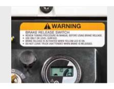
**Drive/Tow Switch** Electronically releases the parking brake to allow a disabled truck to be moved to
