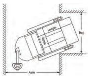
Aisle dimensions listed above assume the minimum bay width to be straddle OD plus 5" (2.5" on either side of straddle leg). Straddle OD is the load width plus 10". Truck performance may vary due to application requirments and changes in model design.
